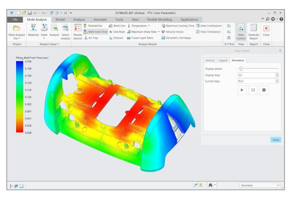
Simulate injection molding process with the Creo Mold Analysis Extension.
